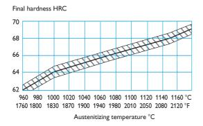
Hardness for different austenitizing temperatures after tempering 3 times for one hour at  $560^{\circ}C$  (±1 HRC).
